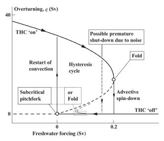
Figure 3.3 A schematic diagram of the thermohaline response showing the two bifurcations and the associated hysteresis cycle (Rahmstorf 2000). The subcritical pitchfork bifurcation will be observed in very simple models, but will be replaced by a fold in more elaborate ones: see, for example, Figure 3.5(b). Note that 1 Sv is  $10^6$  cubic metres per second, which is roughly the combined flow rate of all rivers on Earth.
