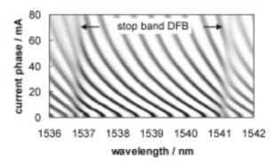
Figure 6: ASE measured at the amplifier facet with the DFB section pumped at transparency. The cavity between end-facet and DFB grating allows for a verification of the phase shift in the passive section. The excess loss by free carrier injection causes the damping of the ASE modulation with increasing current.
